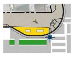
**Plan** - Typical bulb-out seating and paving locations shown in yellow (two locations total).
